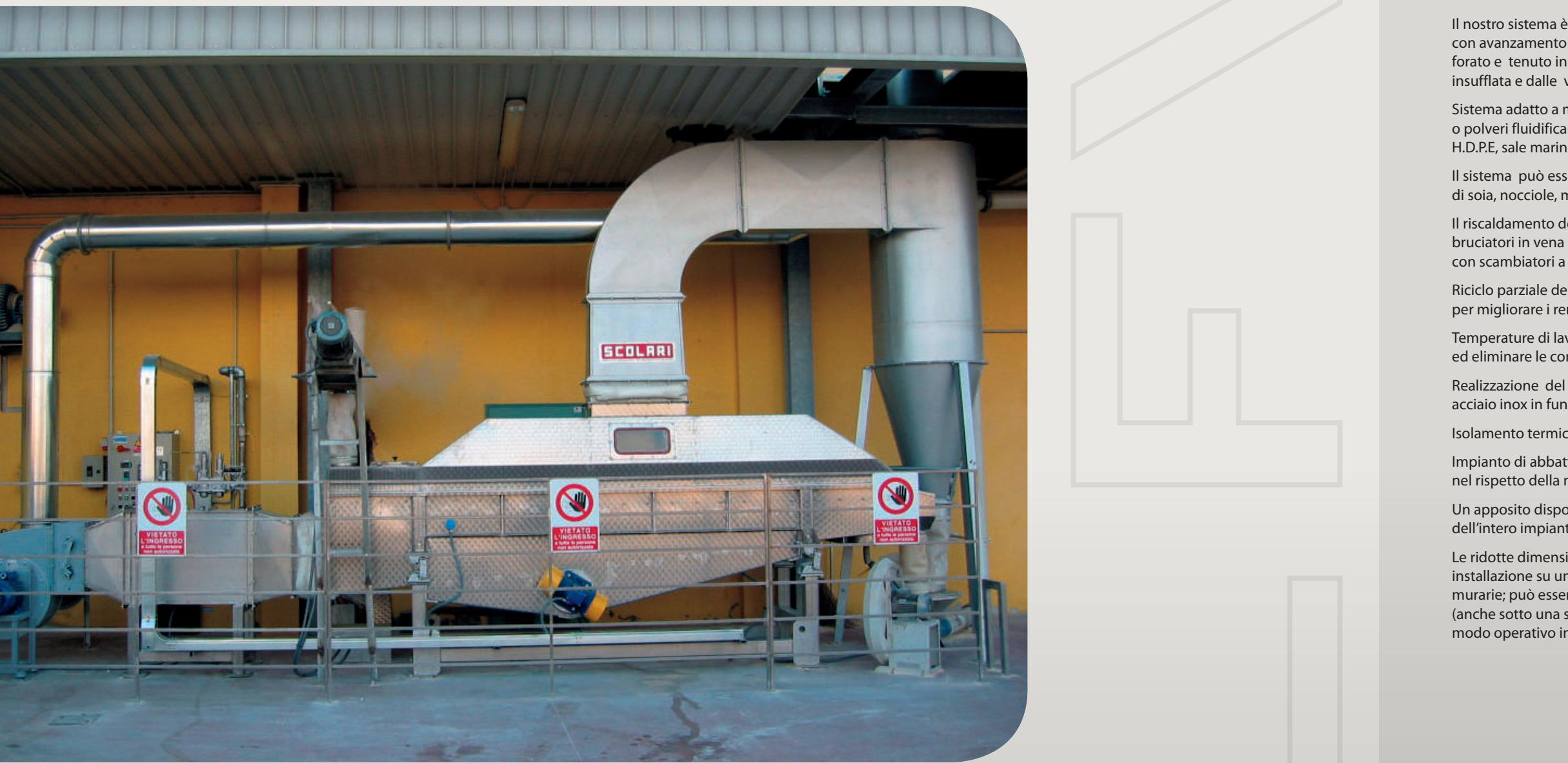
Our system is based on the principle of the fluid vibrating bed with advancing of the material on a surface particularly perforated and kept in suspension by the directional flux of the insufflated air and the
